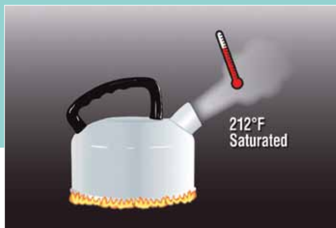
Image 1 This illustration is a basic example of the definition of saturation temperature—the temperature at which fluid boils.
