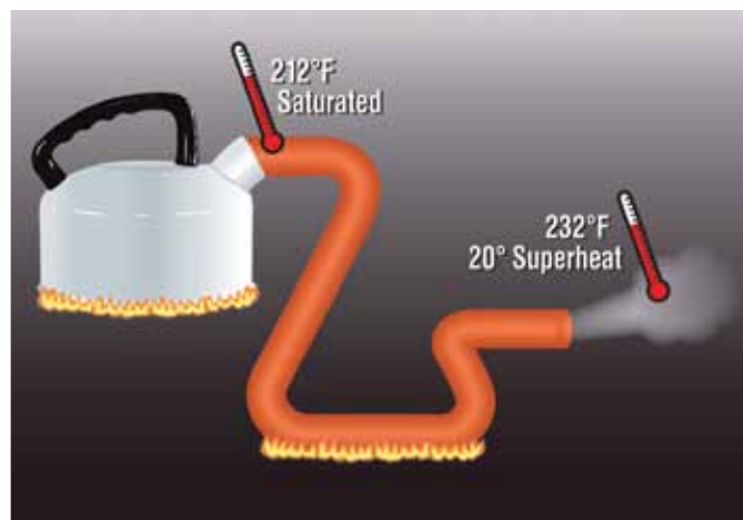
Image 2 The addition of heat to saturated steam (as illustrated above) superheats the steam's temperature.
